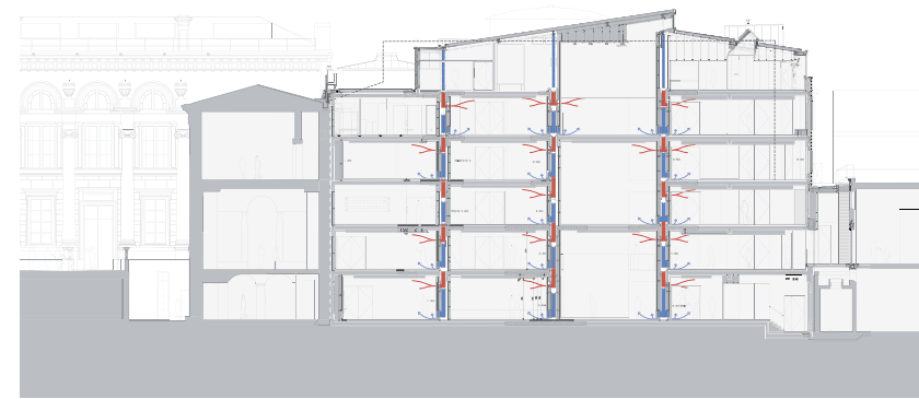
The Ashmolean Museum extension with innovative “fat walls” that carry all of the services in the building
