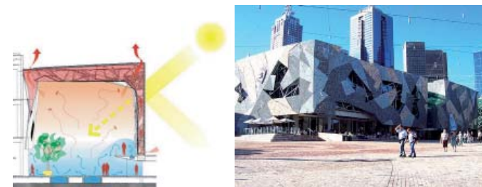
Atelier Ten were the sustainability consultants on Federation Square in Melbourne. Section the atrium of the building with diffusion and passive ventilation strategies and the resulting reduction of unwanted solar gain
